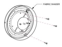
Fasten the steel plate to wall with min. 3 anchors. Use the central slote holes for additional anchors.
